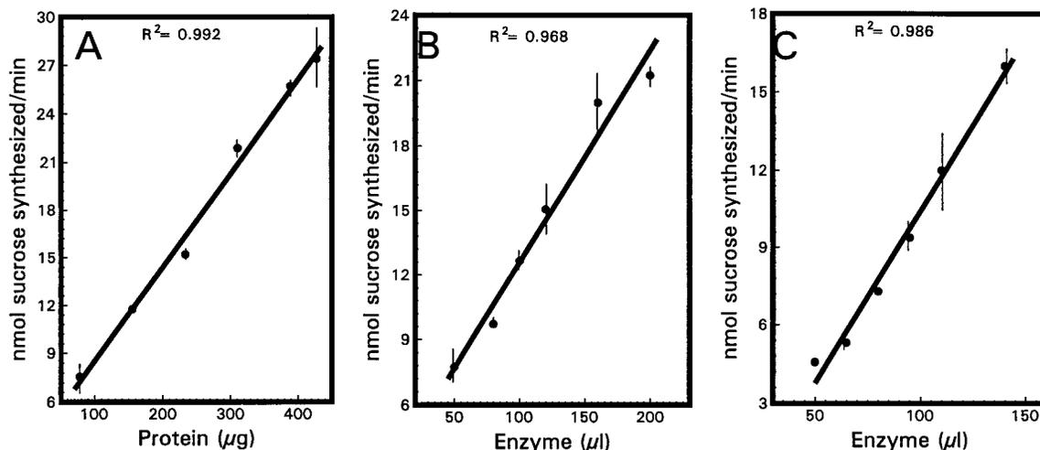
**Figure 7.** Enzyme concentration dependence of SS assay in 50 mM HEPES/KOH/10 mM  $K_2HPO_4$  buffer: (A) purified sucrose synthase from wheat germ; (B and C) partially purified SS preparations from muskmelon fruit and sweetpotato roots, respectively. Each data point was the mean of four replications. Vertical bars represent the standard error.
