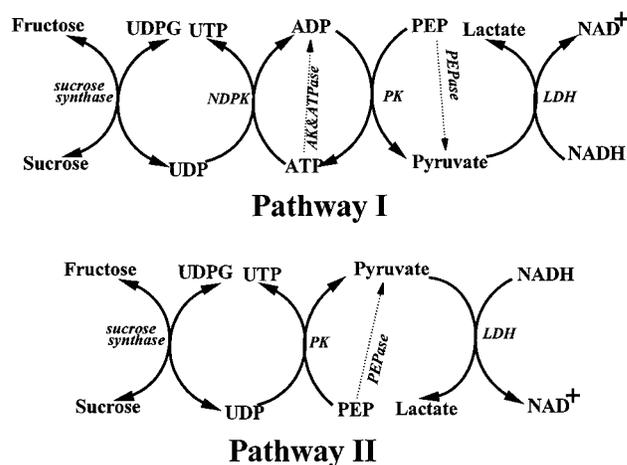
**Figure 1.** Schematic diagrams of the PK/LDH system for SS assay. Pathway I is the modified PK/LDH system by inclusion of ATP and NDPK. The broken lines indicate the interfering enzymes leading to blank rates of NADH oxidation.
